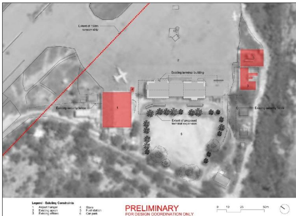
Figure 4 TRW Terminal and Apron Precinct Constraints Plan
