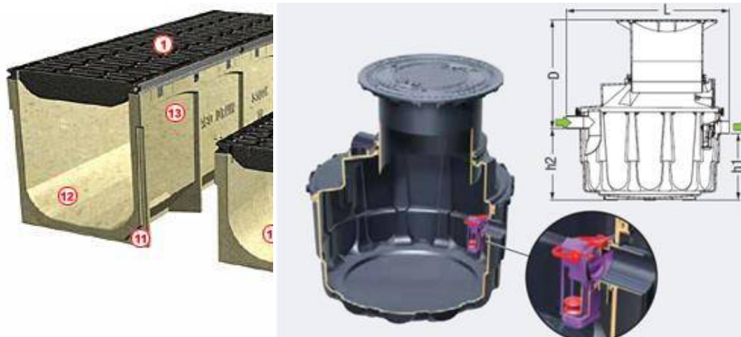
Figure 2 Diagrams of typical preformed slot drain units & an example of the proposed oil separator pod
